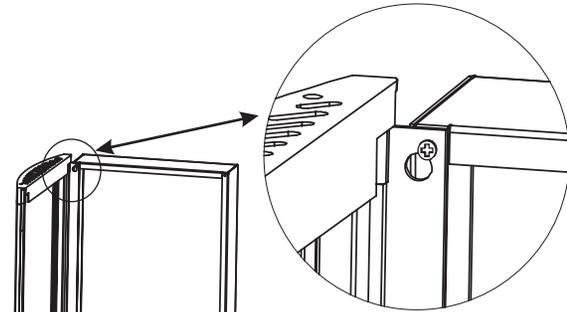
2. Install screws in the middle and bottom of hinge. (Note: C-0128D does not have a bottom screw)
