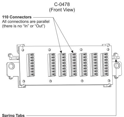
Press into mounting holes in Channel Vision's structured wire enclosure
