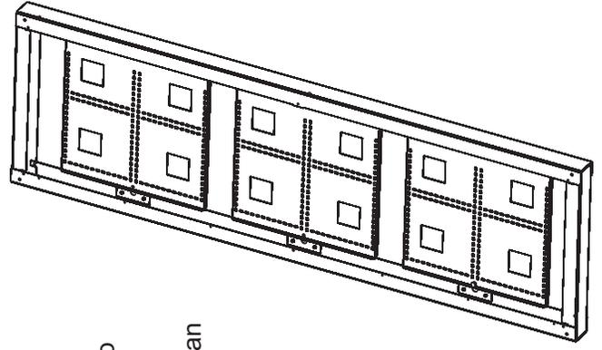
The 50" extension ring can hold up to three C-1321 as shown.
