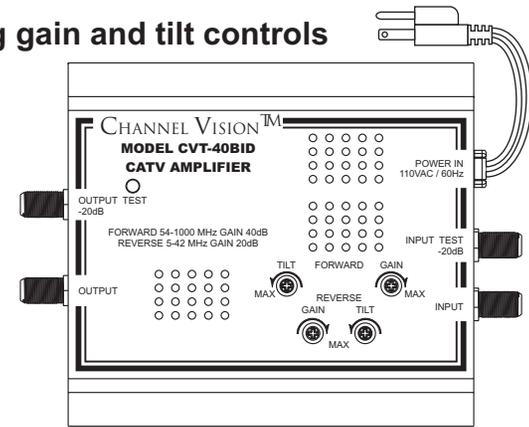
**Gain control ...** The gain control is a variable attenuator that will reduce the level of the signal before the gain stage of the CVT-40BID. The number one problem with video distribution systems is inter-modulation (IM) distortion caused by over driven amplifiers. The symptom of IM is a herringbone pattern on one or more channels.
