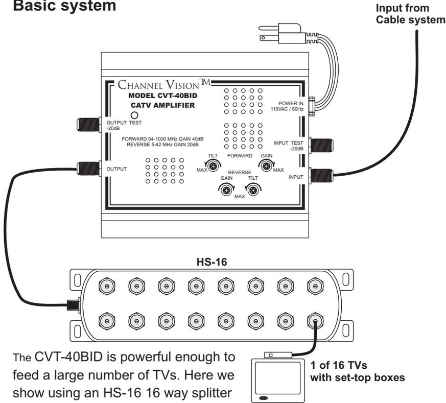
The CVT-40BID is powerful enough to feed a large number of TVs. Here we show using an HS-16 16 way splitter to distribute video in a large house.
